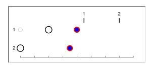
... so cell 1's trajectory isn't affected. There are no events between its current time t\_ and tn, so t\_ can be moved right up to tn, as shown here. Technically speaking this is an "interpolation" even though no real calculations are involved.
