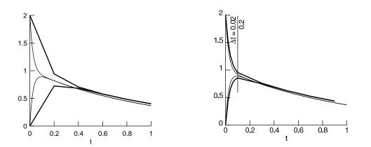
Figure 4.6. Simulation of the two compartment model of Fig. 4.4 using the backward Euler method. Left:  $\Delta t = 0.2$  s, much larger than the fast time constant. Right:  $\Delta t$  was initially 0.02 s, small enough to follow the first time constant closely. After 0.1 s,  $\Delta t$  increased to 0.2 s but the solution remained stable. Thin lines are analytic solution, thick lines are backward Euler solution. Modified from (Hines and Carnevale 1997).
