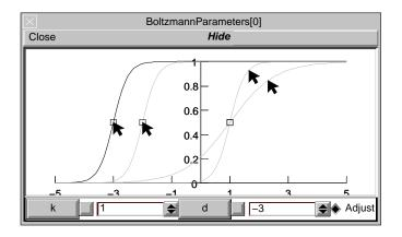
Fig. 14.6. Final appearance of the "Boltzmann Parameters" tool. The parameter values displayed are for the leftmost curve. Other curves with arrows suggest the process of selection and dragging the mouse.
