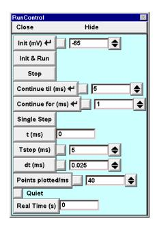
Figure 1.30. Left: To bring up a window with controls for running simulations, click on the RunControl button in NEURON Main Menu / Tools. Right: The RunControl window provides many options for controlling the overall time course of a simulation run. For this example, only three of these controls are relevant.
