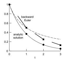
Figure 4.5. Comparison of analytic solution to Eq. 4.19 (solid line with circles) with results from the backward Euler method (Eq. 4.25, squares) for V(0) = 1, k = 1/s, and  $\Delta t = 1$  s. At the end of each step, the slope at the new value (heavy lines) points back to the beginning of the step. The dashed line shows the voltage after the first time step as a function of  $\Delta t$ . Modified from (Hines and Carnevale 1997).
