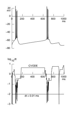
burst (Fig. 4.13). The remarkable speedup by CVODE is due to the fact that  $\Delta t$  was much larger than 0.01 ms for most of the simulation.
