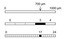
Figure 5.4. Boxed in by compartments. Top: Conceptual model of an unbranched axon 1000  $\mu$ m long. We are interested in membrane potential at a point 700  $\mu$ m from its left end. Middle and bottom: The index of the compartment that corresponds to the location of interest depends on how many compartments there are.
