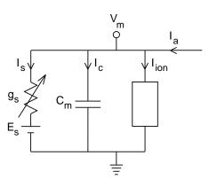
Figure 10.1. Membrane potential in the immediate neighborhood of a postsynaptic conductance depends on the synaptic current  $(I_s)$ , the currents through the local membrane capacitance and ionic conductances  $(I_c \text{ and } I_{ion})$ , and the axial current arriving from adjacent regions of the cell  $(I_a)$ .
