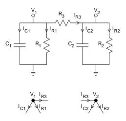
Fig. 3.5. Top: A circuit with three nodes. Bottom: Current flow diagram at each of the two nodes where potential is unknown. Note the direction of current flow in  $R_3$ .
