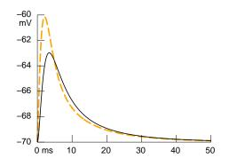
Figure 5.11. Time course of  $V_m$  at the synaptic location. The dashed orange line is the analytic solution, and the solid black line is the numeric solution computed with  $\Delta t = 1 \ \mu$ s. Modified from (Hines and Carnevale 2001).
