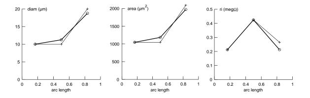
Figure 5.8. diam, area, and ri at the internal nodes of a 100  $\mu$ m long section with nseg = 3 and Ra = 100  $\Omega$  cm. Thin lines with + show the values immediately after geometry was specified, when no 3-D points existed. Thick lines with circles show the values after define\_shape() was executed, creating a set of 3-D points and forcing recalculation of diam, area, and ri.
