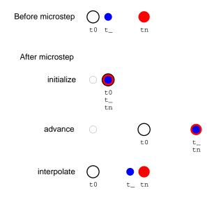
Fig. 7.2. After a microstep, the relative positions of  $\pm 0$  (black open circle),  $\pm$  (blue dot), and  $\pm n$  (red filled circle) in time depends on whether the microstep performed an initialization, a normal integration step, or an interpolation to just before the next event. The small grey circle after initialize and advance marks the former location of  $\pm 0$ . Time increases toward the right in each row.
