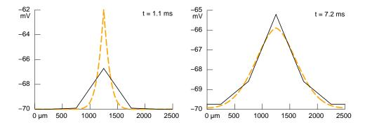
Figure 5.12.  $V_m$  vs. distance along the dendrite computed during the rising (left) and falling (right) phases of the EPSP. The analytic and numeric solutions are shown with dashed orange and solid black lines, respectively. The error of the numeric solution is greatest in the region where  $V_m$  changes most rapidly, i.e. in the neighborhood of the synapse.
