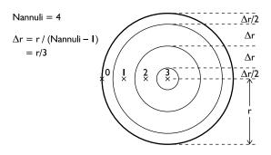
Figure 9.9. Diagram of the concentric shells used to model radial diffusion. The  $\times$  mark the radial distances at which concentration will be second order correct in space.
