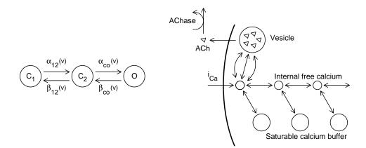
Fig. 3.1. Left: a voltage-gated channel modeled as a three-state kinetic scheme with voltage-dependent rate constants. Right: cartoon of a model of acetylcholine (ACh) release that involves the influx, buffering, and diffusion of calcium, exocytosis requiring binding of three calcium ions per vesicle, and enzymatic breakdown of ACh (rate constants omitted for clarity).
