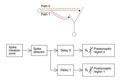
Figure 10.5. Efficient divergence. Top: A single presynaptic neuron projects to two different target synapses. Bottom: Computational model of this circuit uses multiple NetCons with a single threshold detector that monitors a common source.
