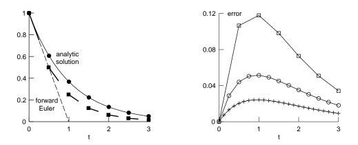
Figure 4.3. Left: analytic solution to Eq. 4.19 (solid line with circles) and results of the forward Euler method (squares) for V(0) = 1, k = 1/s, and  $\Delta t = 0.5$  s (modified from (Hines and Carnevale 1997)). Right: absolute error of the forward Euler method with  $\Delta t = 0.5$  (squares), 0.25 (circles), and 0.125 s (+).
