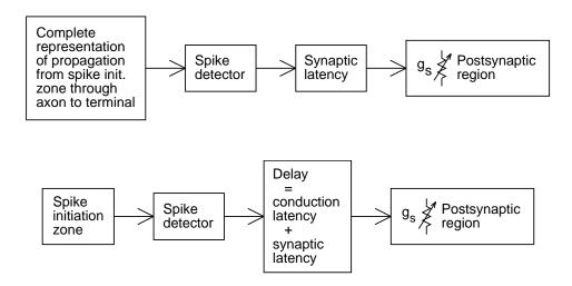
Figure 10.4. Computational implementation of a model of spike-triggered synaptic transmission. Top: The basic idea is that a presynaptic spike causes some change in the postsynaptic cell. Bottom: A more efficient version doesn't bother computing conduction in the presynaptic axon.
