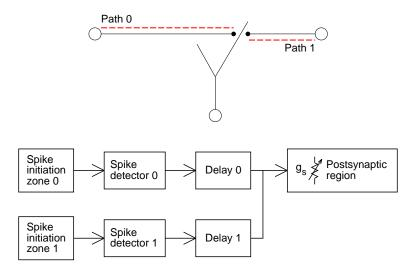
Figure 10.6. Efficient convergence. Top: Two different presynaptic cells make synaptic connections of the same class that are electrically close to each other. Bottom: Computational model of this circuit uses multiple NetCons that share a single postsynaptic mechanism (single equation handles multiple input streams).
