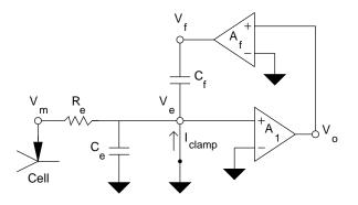
Fig. 3.6. Capacitance compensation under current clamp. The capacitance  $C_e$  of the microelectrode distorts recordings by slowing and attenuating the response of  $V_e$  to changes in  $V_m$  and  $I_{clamp}$ . Amplifier  $A_f$  and capacitor  $C_f$  compensate for this by supplying charging current to  $C_e$ .
