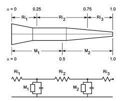
Figure 5.7. Representation of the neurite of Fig. 5.6 when nseg = 2. The equivalent circuit now has two nodes. See text for details. Reproduced from (Hines and Carnevale 1997).
